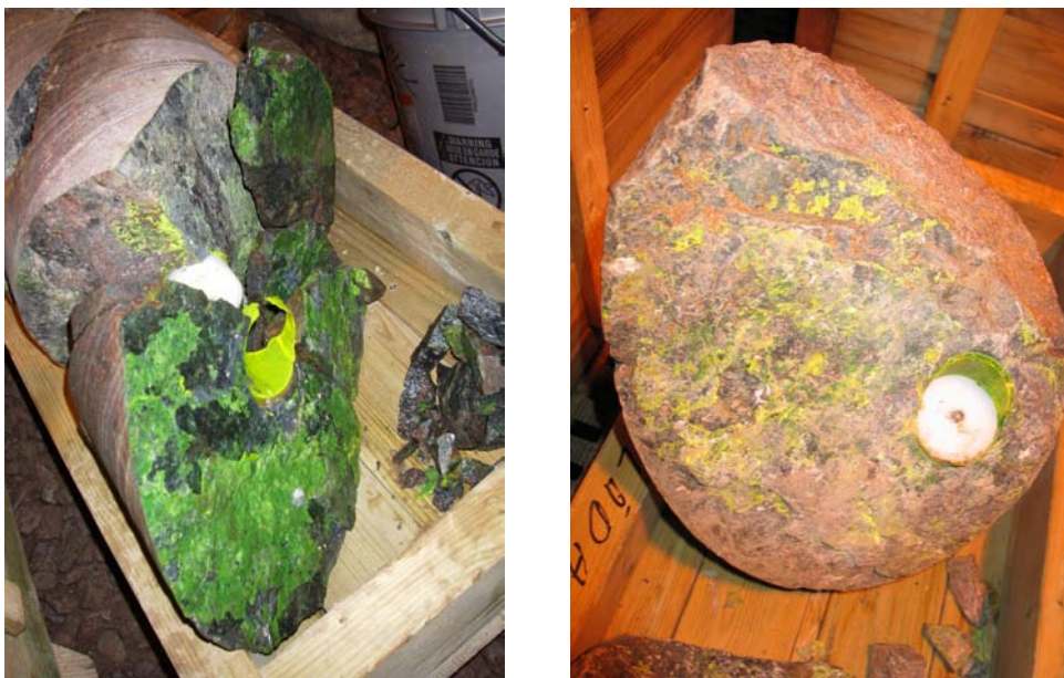
Figure 3-2. Feature A in KXTT3 (to the left) and in KXTT4 (to the right). The green material is uranine tagged epoxy.
