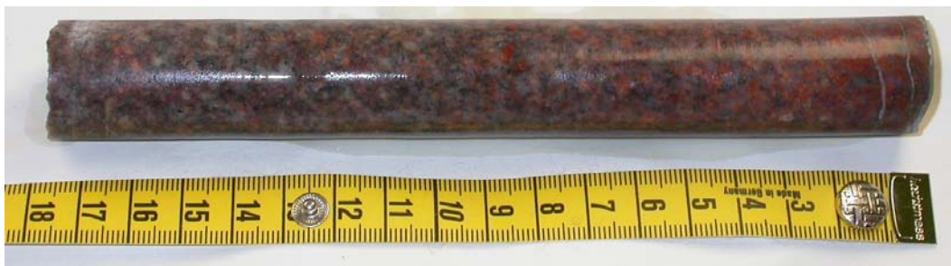
Figure 3-3. Sample core A6, about 18 cm long, drilled from the fracture surface on the core stub. Underneath the protective coating of epoxy resin a thin layer of calcite and chlorite is seen on the fracture surface. The rock is altered into about 4 cm from the fracture surface. Close to and in parallel to the fracture surface two fractures sealed with calcite are visible.
